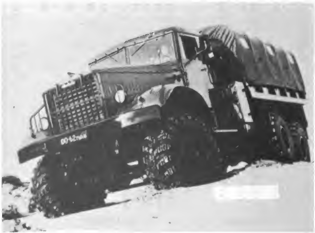
Figure 6-73. Heavy trucks. The 7.5-ton KrAZ-255B (above) is often used to carry bridge spans for the PMP folding bridge. The MAZ-535 (below) tows a launcher/trailer for surface-to-air missiles.
